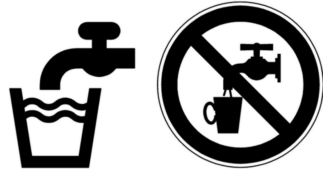
Figure 6 — Signs "Potable water" (left) and "Non-potable water" (right) according to EN 806-2
